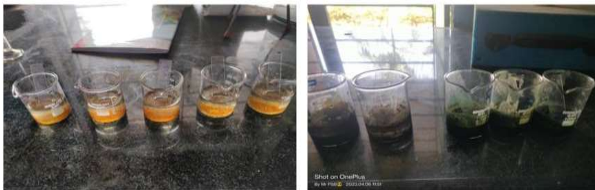
Fig 1.1 and 1.2 before oxidation and after oxidation the formation Biocomposites films of PANI-Ni NPs.
